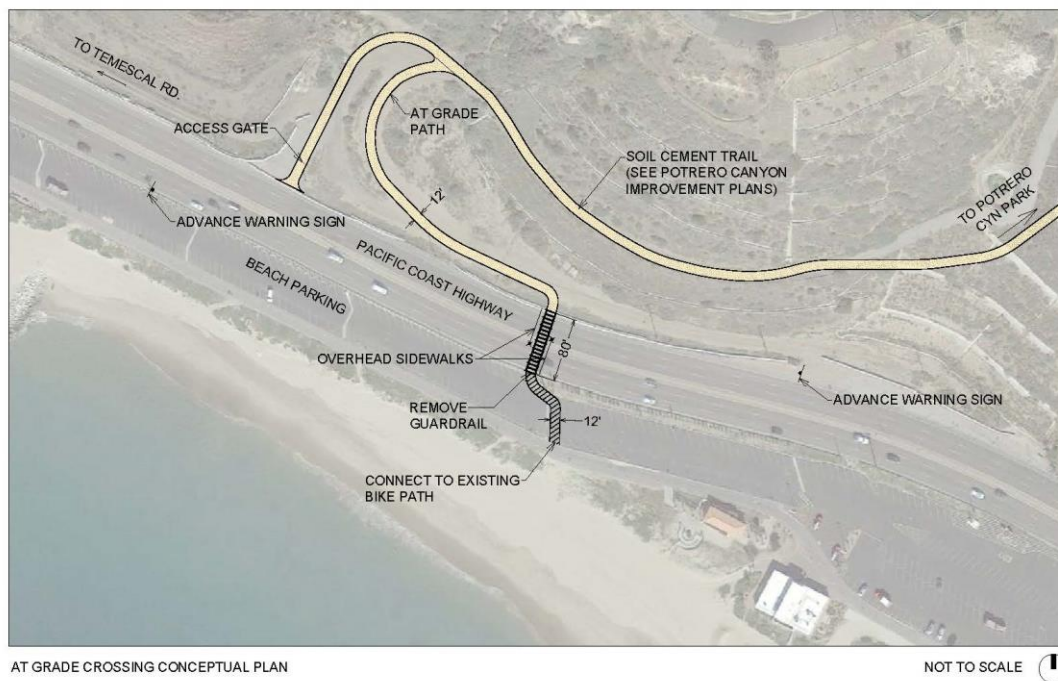
Figure 3. At-Grade Crossing Layout
