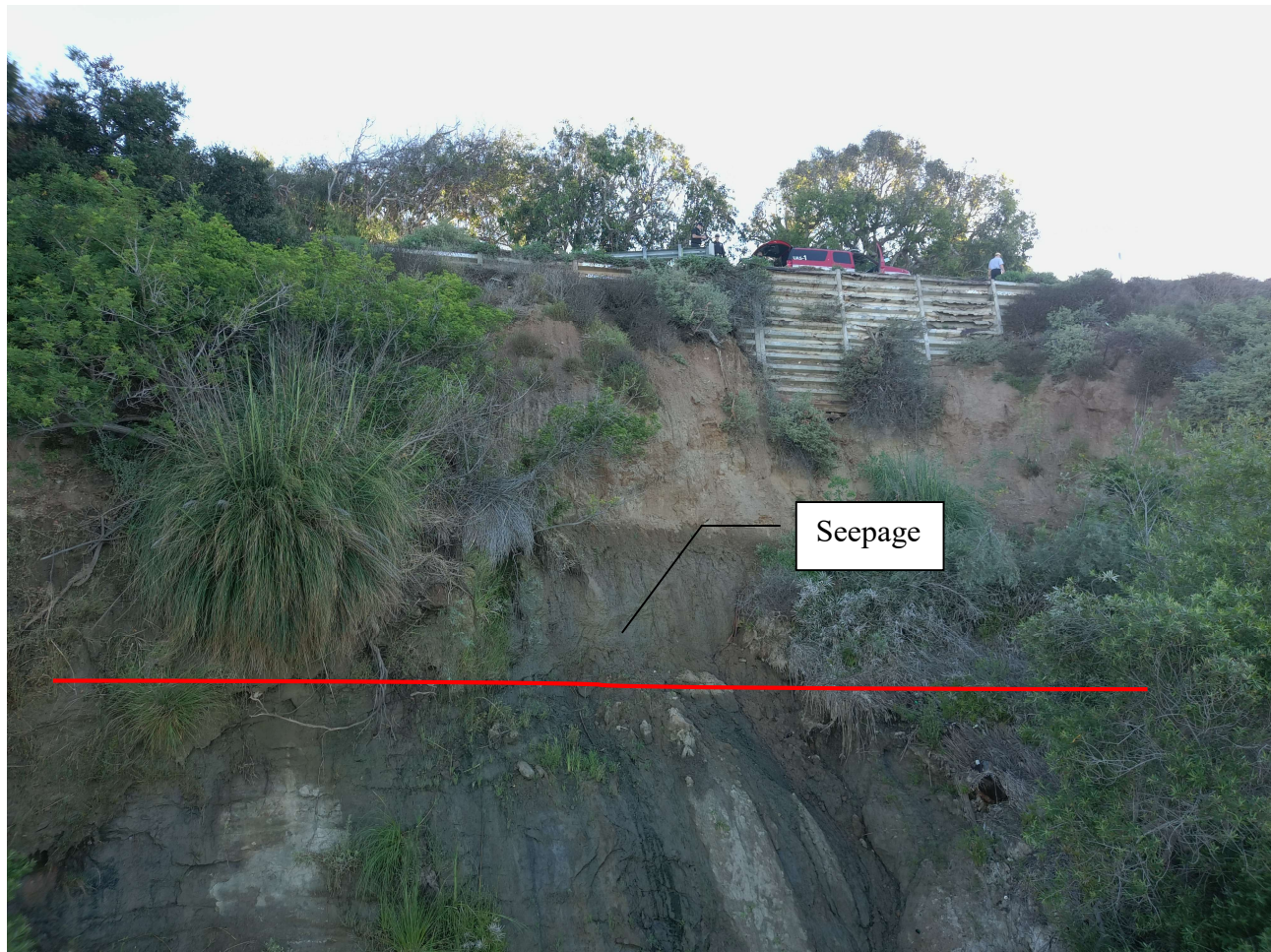
Photo 2: An August 30, 2023 LAFD aerial drone image shows a closer image of the head scarp of the slide. The geologic contact is outlined in red. Groundwater which has reached the surface emanates as a spring, where the alluvial terrace overlies the less permeable siltstone Fernando formation below.
