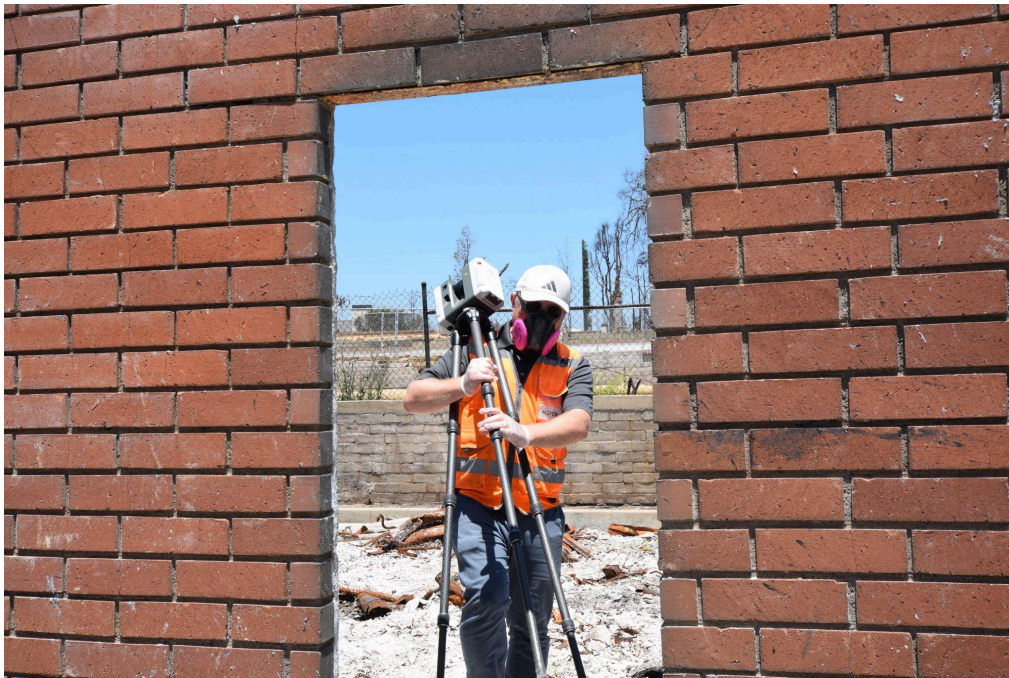
Alan White, Principal at AQYER, carries a Leica RTC360 Laser Scanner in the Pacific Palisades. Photo © Morgan Richmeier, AQYER, LLC
